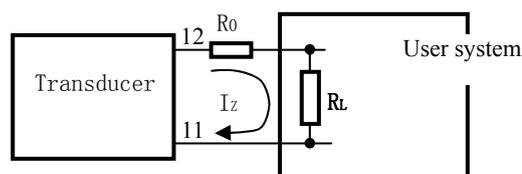
3. basic testing method for accuracy
