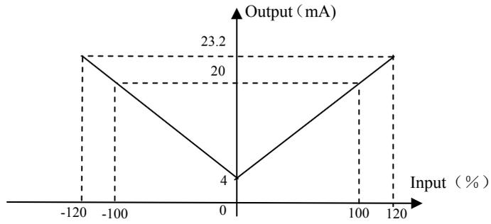
4mA~20mA Input-Output characteristic curve
