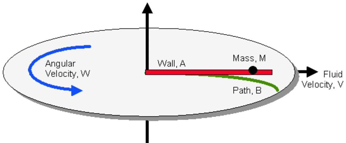
If the mass M is guided by Wall A (i.e. the tube), a Coriolis Force will be exerted on the wall as shown below.
