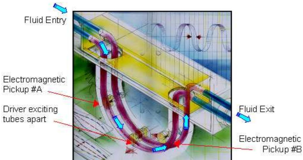
The tube walls guide the process fluid as it flows through the U-Tube pathway. With no fluid inside the tubes the Driver excites the tubes apart at a nominal 150Hz as shown below.
