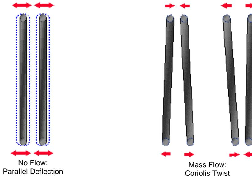
Now imagine fluid of Mass M flowing through and out of the RotaMASS tubes. As the fluid flows down the first half of the U-Tubes it will tend to deflect the tubes in towards each other. Conversely, when the fluid flows up the second half of the U-Tubes it will tend to deflect the tubes out away from each other. This Coriolis Twist action is shown above.
